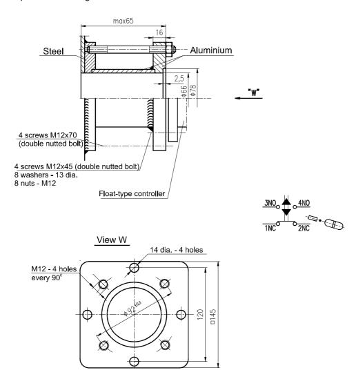
Manufacturer recommends to weld connecting flange directly to tank (without socket ferrule)
