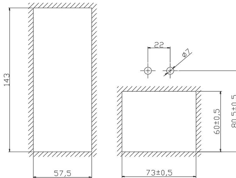
a) the hole in the table for assembly – for standard regulator
