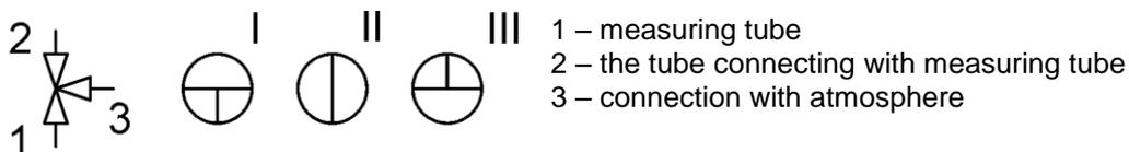
Drawing no. 9. Three-way manifold
