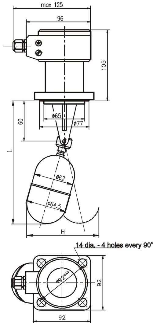
Dimension drawing of level switch type ERH-01-04 with cranked arm
