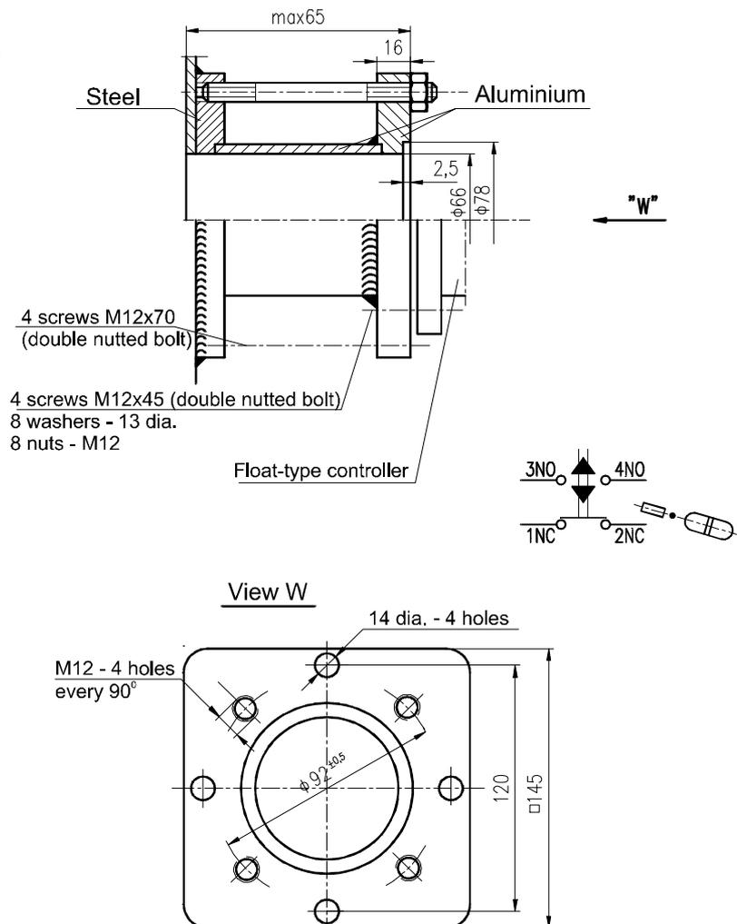
**Manufacturer recommends to weld connecting flange directly to tank (without socket ferrule)**
