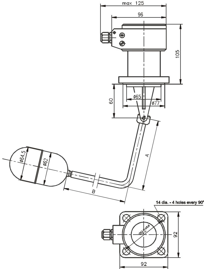
Dimension drawing of level switch type ERH-02-04
