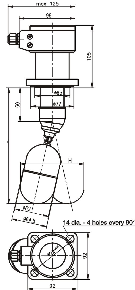
Dimension drawing of level switch type ERH-03-04
