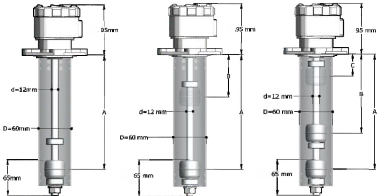
The dimensions A, B and C depend on the ordered version. For one signalling point: A min. 50mm, A max. 1000mm. For two signalling points: A min. 150mm, A max 1000mm; B min. 50mm, B max 900mm; (A – B) min. 100mm. For three signalling points: A min. 250mm, A max 1000mm; B min. 150mm, B max 900mm; C min. 50mm, C max 800mm; (A–B) min. 100mm, (B–C) min. 100mm.
